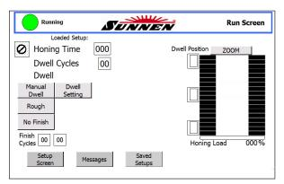
Easy-to-read and use bore profile display takes the guesswork out of removing taper.
