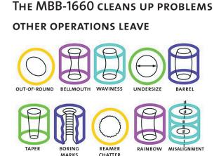
There are ten common bore errors that are caused by machining, heat treat or chucking. All of them can be corrected quickly and easily on the Sunnen MBB-1660.
