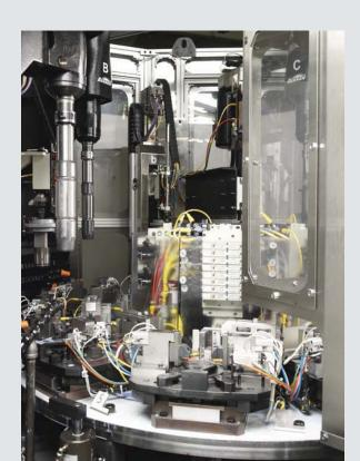
Our fixturing, automation and other customization options are designed to increase the operational efficiency of your precision honing system while significantly reducing labor costs. From integrated air gaging to robotic work-piece handling, Sunnen solutions can be customized to satisfy the requirements of even the most specialized applications.
